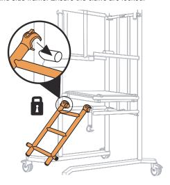
Rotate the ladder down, using the claws as pivots. Locate the bottom of the ladder over the base frame as shown below.
