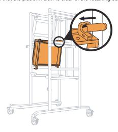
Rotate the platform down and locate the platform claws on the horizontal member of the right hand side frame. Push the platform back towards the back of the unit until it is in contact with the rear folding guardrail frame. Ensure the claws are sitting on the tube and not the plates.
