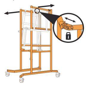
4 Slide the platform towards the front of the unit (the open end) so that the platform claw is clear of the retaining bar.
