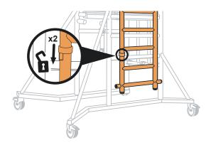
Locate the ladder claws over the spigots on the left and right hand side frame. Ensure the claws are locked.
