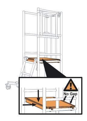
Push the platform towards the back of the unit until it is in contact with the rear folding guardrail frame. Lock the platform retaining plates.
