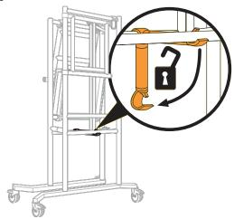
Open the side frames, which will allow the rear folding guardrail frame to unfold. Ensure the rear folding frame is fully open and both elbow joints are locked.
