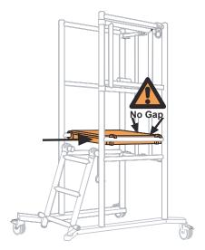
Using the ladder section, climb onto the platform of the work station.
