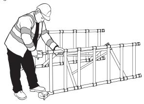
When using adjustable legs for uneven or sloping ground, push 4 castors into 4 adjustable legs and then insert the adjustable legs into the bottom of the base unit. The bottom of the base unit may be identified by the bottom end casting - see diagram.
