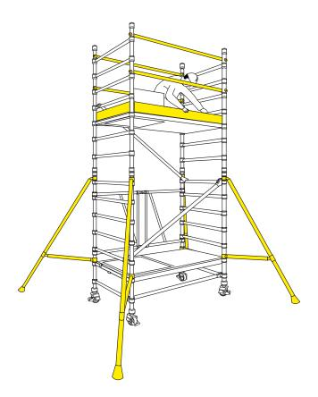
IMPORTANT. Always ensure braces are fully locked in position.
