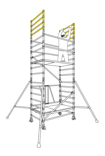
6 The platforms must now be repositioned as follows: Whilst standing on the upper deck, unlatch the 4 guardrail brace hooks furthest from the trapdoor but leave the braces in position. From the protects position of the trapdoor deck, unlatch the remaining 4 brace hooks and remove the 4 guardrail braces and then descend immediately to the lower platform.
