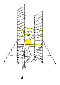
7 Fit a diagonal between the 9th and 13th rungs of the tower. Fit a deck on the 14th rungs of the tower. From the protected position of the trapdoor deck, fit a pair of guardrails 2 and 4 rungs above the platform (16th & 18th rungs of the tower). Fit a diagonal between the 14th and 18th rungs of the tower, as shown.
