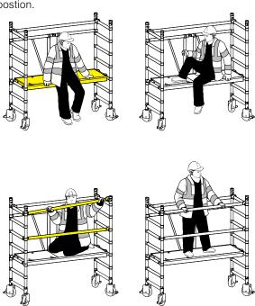
6 If your risk assessment shows it is necessary, fit a set of toeboards to the platform. Check there are no gaps through which any materials could fall and that the trapdoor opens correctly. The tower is now complete.
