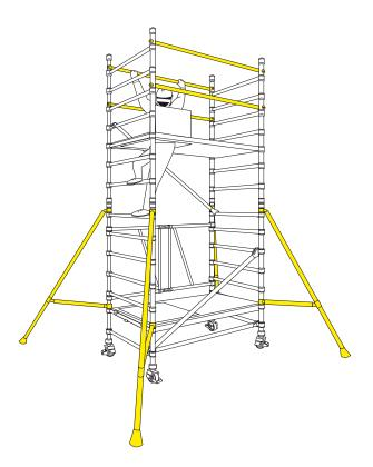
5 Fit a 4 rung guardrail frame to each end of the tower. Ensure the frame interlock clips are engaged.
