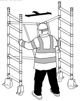
Check the ground is flat and all four castor wheels are in contact with the ground.
