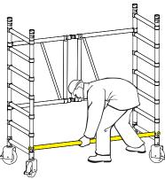
3 Position a temporary platform on the 2nd rungs of the tower. Engage the wind locks, underneath the rungs, at both ends of the platform.
