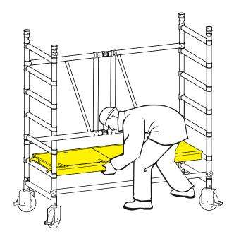
3 Fit a 7 rung lift frame to each end of the base unit. Ensure the 4 frame interlock clips are engaged.
